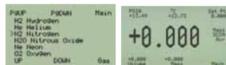
Meters and controllers feature a dynamic display that simultaneously shows flow rate, line pressure, fluid temperature, and (for controllers) the set point. For the units shown, both power and input/output signals are transmitted through a single multi-pin connector.
